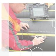
The need to guarantee the integrity of the base material of structural and engineered plastic piping and engineering such as HDPE and PVC, coupled with the need to detect or prevent defects during the welding process, whether by thermal-fusion or electro-fusion, led NDT Innovations to search for new procedures for inspecting these materials.
