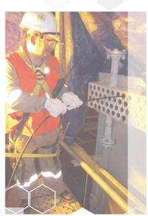
NDT Innovations uses electromagnetic inspection technologies focused on measurement. NDT Innovations is capable to provide inspection support and guarantee of integrity for mining equipment in typically short timeframes during maintenance shutdowns. The versatility of the methods we apply allows us to achieve a flaw detection capacity even over thick layers of paint, or lubrication grease of moving components (such as gears, mills, chassis, conveyors, among other components).
