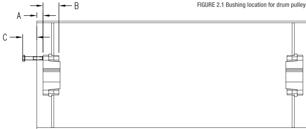
FIGURE 2.1 Bushing location for drum pulleys
